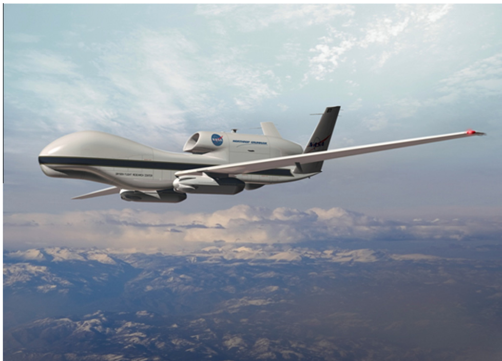
Fig. 2. Artist's concept of the Global Hawk UAS with proposed dual antenna UAVSAR system installed.
