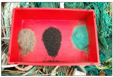
Used fishing nets are a growing environmental problem, because up till now it was not possible to recycle them effectively. The plant from Frandsen Industri, however, can shred and separate the different plastic types in one process. The black heap in the middle is plastic granulate ready for use and produced from separated and extruded fishing nets. The density of the material can be adjusted.
